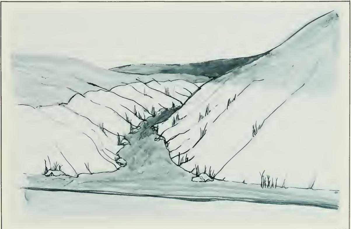
Lay-back draw; cut slope flattened to match slope of draw
