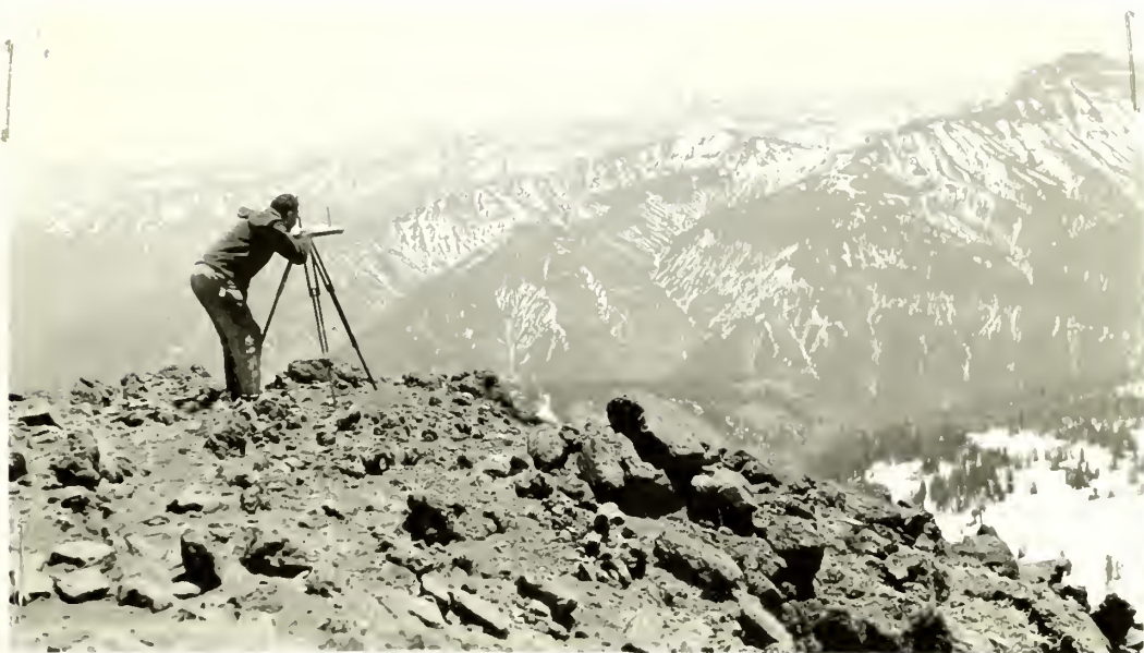
Mapping timber types by use of plane table from top of Saddle Mountain. Note quantities of snow as yet unmelted in high areas. Type mappers often required to use snowshoes to attain high peaks for plane table observations and mapping.
