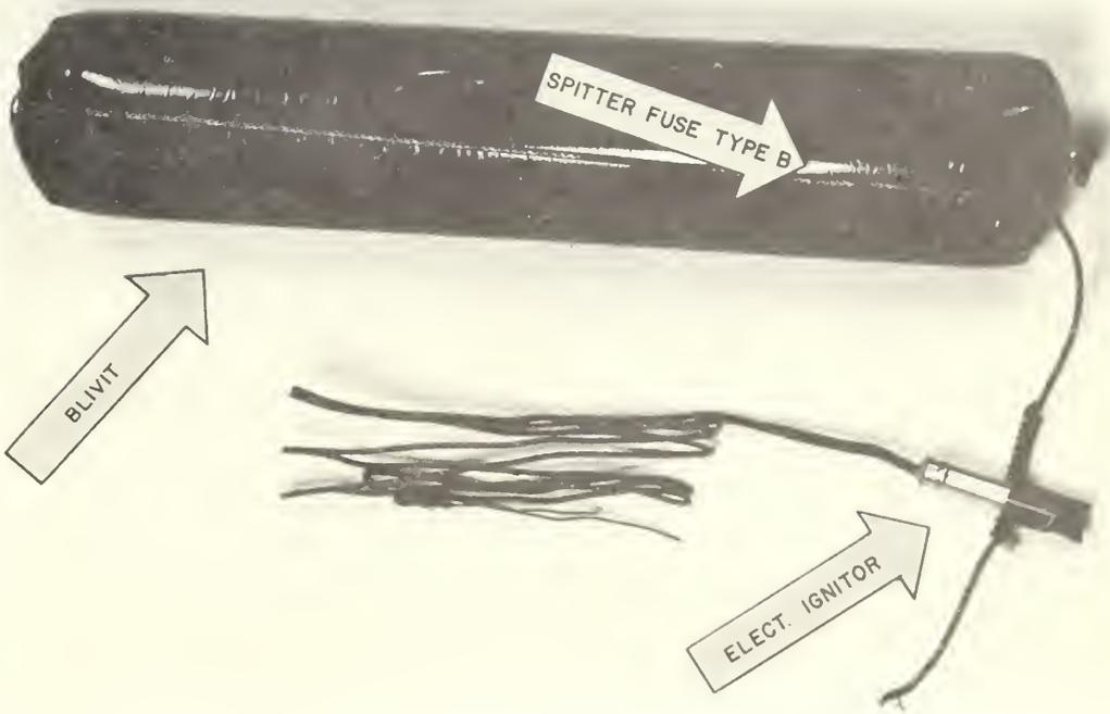
Figure 16.--Jellied diesel oil ignitor.
