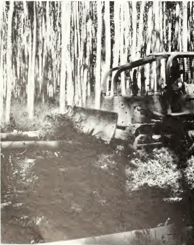
Figure 5.—Regeneration by bulldozing. Stems must be tipped out of the ground. Cutting through soil with the blade will destroy the lateral root system.
