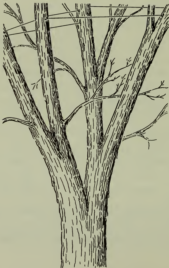
Figure 3.—Triangular cabling system.
