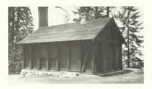
During the 1930s the six-year plans for Lodgepole and Giant Forest called for buildings with "heavy frame type" construction such as that seen here in the Last Hill dormitory. The rubble-veneer foundation, thick structural members, and roof shingling pattern developed into a consistent style for comfort stations and small utilitarian structures.
