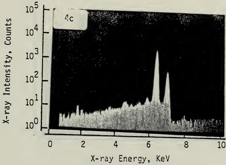
Figure 4c&d. XES Microanalysis Spectra from Piece A (Please see Figure 3a)
