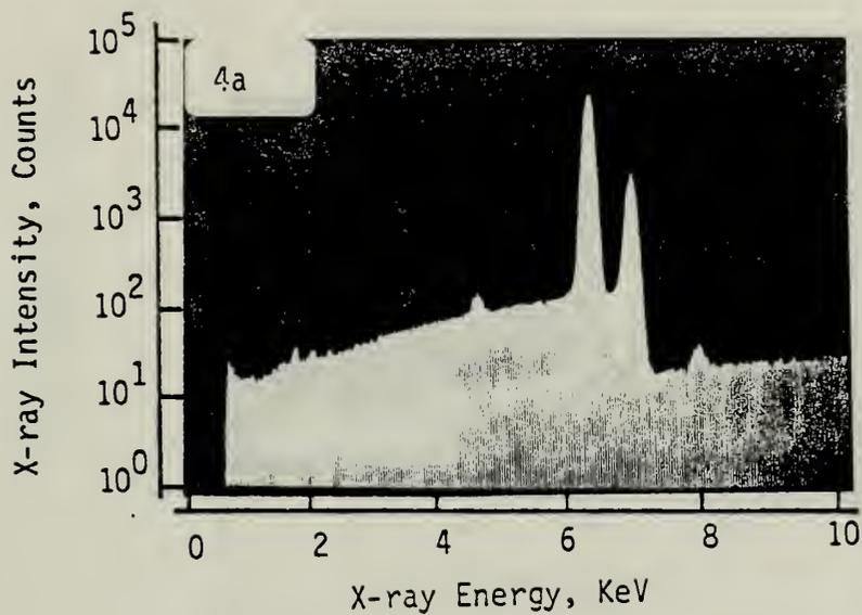
Figure 4a&b. XES Microanalysis Spectra from Piece A (Please see Figure 3a)
