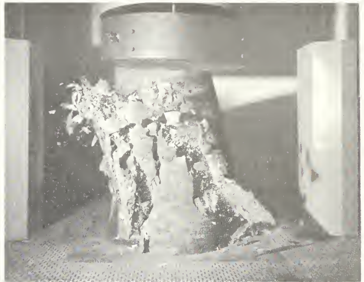
JUST TESTING! —This is the "small" 4,000,000-pound capacity testing machine shattering a concrete core at the Denver Engineering Center. At the dedication ceremonies on July 20, the new 5,000,000-pound capacity testing machine—the last word in machinery for testing concrete and steel—will be shown, ready for use. It took a year to install the jumbo-size equipment.
