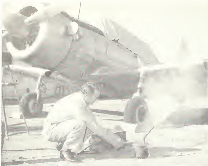
TESTING RAIN "SEED" —C. S. (Chuck) Barnes tries out a metallic sodium generator before installing it in the powerful plane used in seeding rain clouds. Barnes is president of Precipitation Control, Inc., of Phoenix, Ariz., and considers this the newest thing in rainmaking.
