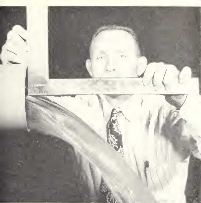
HERE'S AN ANGLE —Upper left: Here is how you use a carpenter's rule to measure the amount of water flowing through a pipe. Upper right: WATCH THE FREEBOARD! Read how it's done and see figure 3 on the next page.
