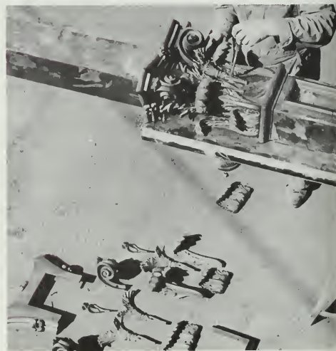
Figure 173. Preassembly of Cast-Iron Components. Before the cast-iron pieces are shipped from the foundry to the job site, the components are laid out and preassembled to insure proper fit. If the parts do not fit because of burrs, the pieces are machined to remove irregularities. If the parts still do not fit, the rejected parts are recast until all of the castings fit together. Some small ornamental parts may be left together, but most of the larger pieces are disassembled before shipping. All of the castings shown were necessary to produce a Corinthian pilaster. (Walter Smalling, Jr.)
