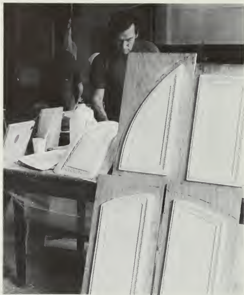
Figure 170. Plastic Patterns. Historically, most patterns for casting iron were carved from wood and pressed into sand to form molds. For the recasting of the iron shutters of the West Virginia Independence Hall, an attempt to use plastic patterns met with only limited success. How the original shutters, with their deeply undercut, beaded molding were cast in one piece is not known. To achieve the same effect in the restoration, the beaded molding of iron had to be cast separately and applied to the replicas. The patterns are mounted on plywood to give them enough rigidity so they may be hammered into the sand to form the molds. (West Virginia Independence Hall Foundation)
