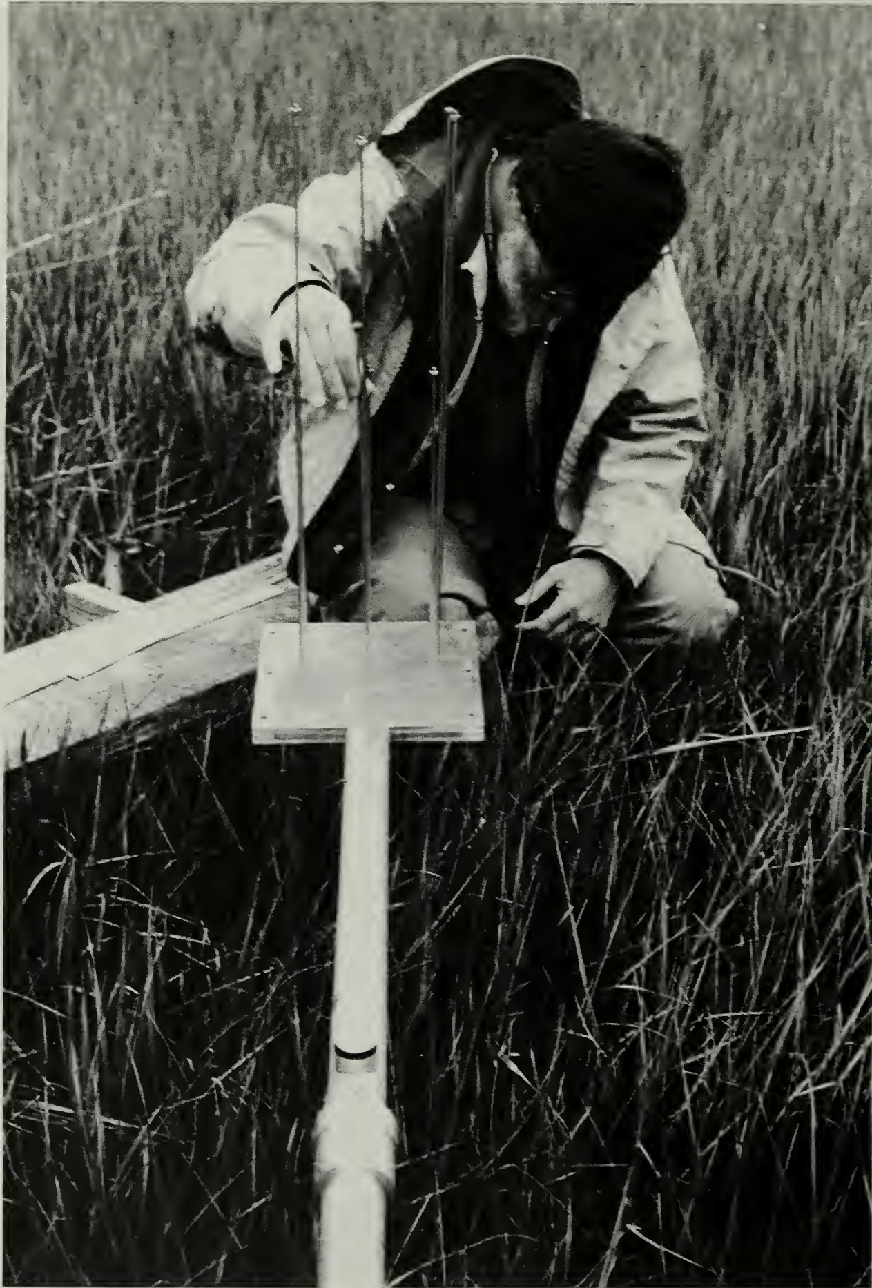
Figure 11. Sedimentation Table Measurements of Marsh Surface
