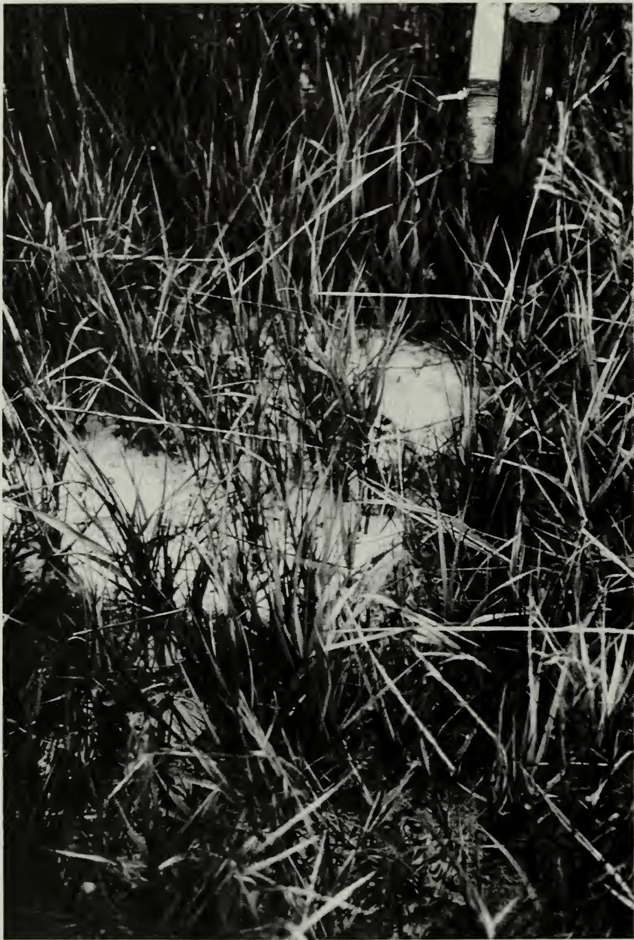
Figure 9. Clay/Feldspar Marker in Marsh
