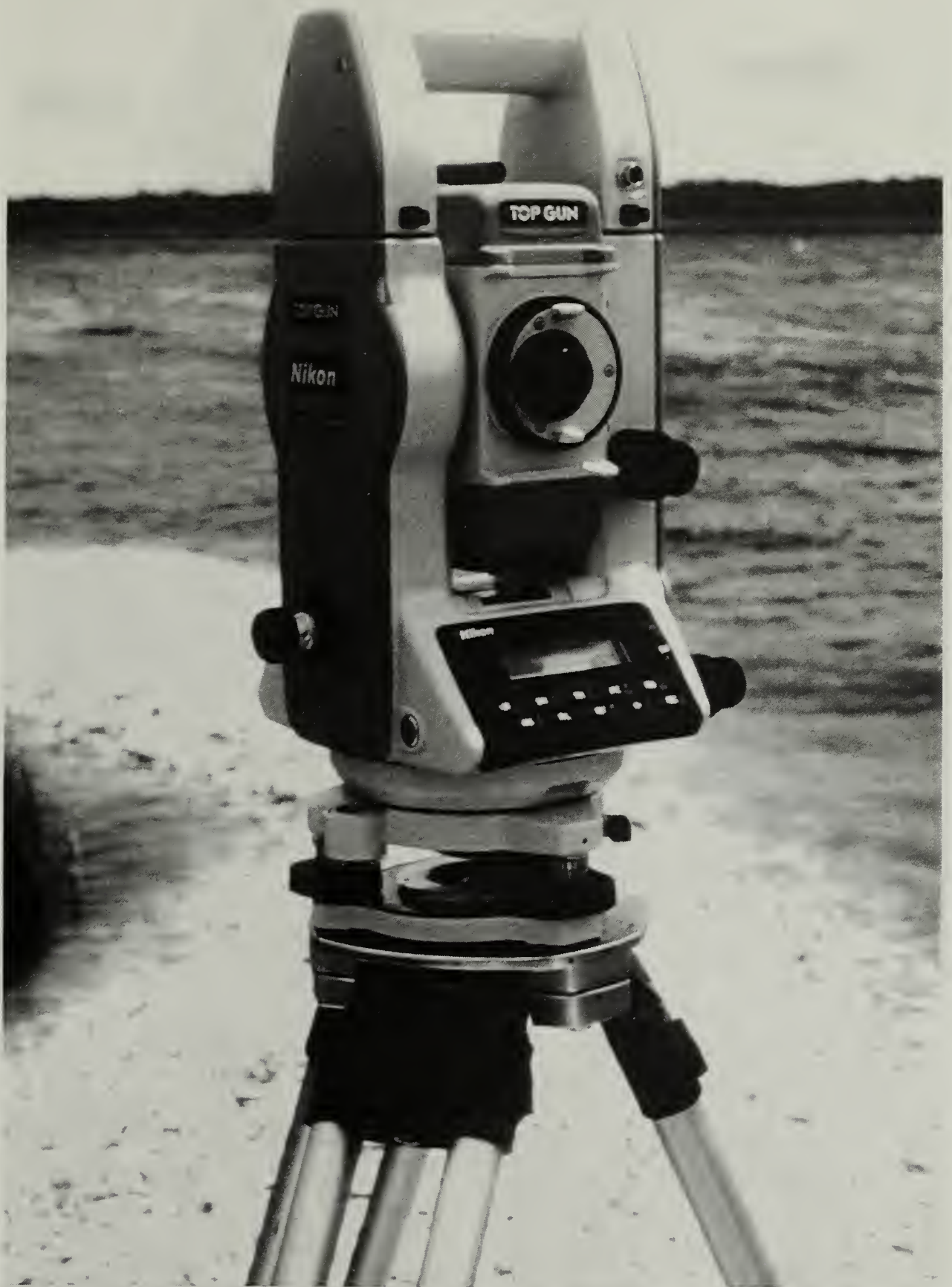
Figure 6. Electronic Distance Meter Unit used to tie-in Subdatums to Benchmarks
