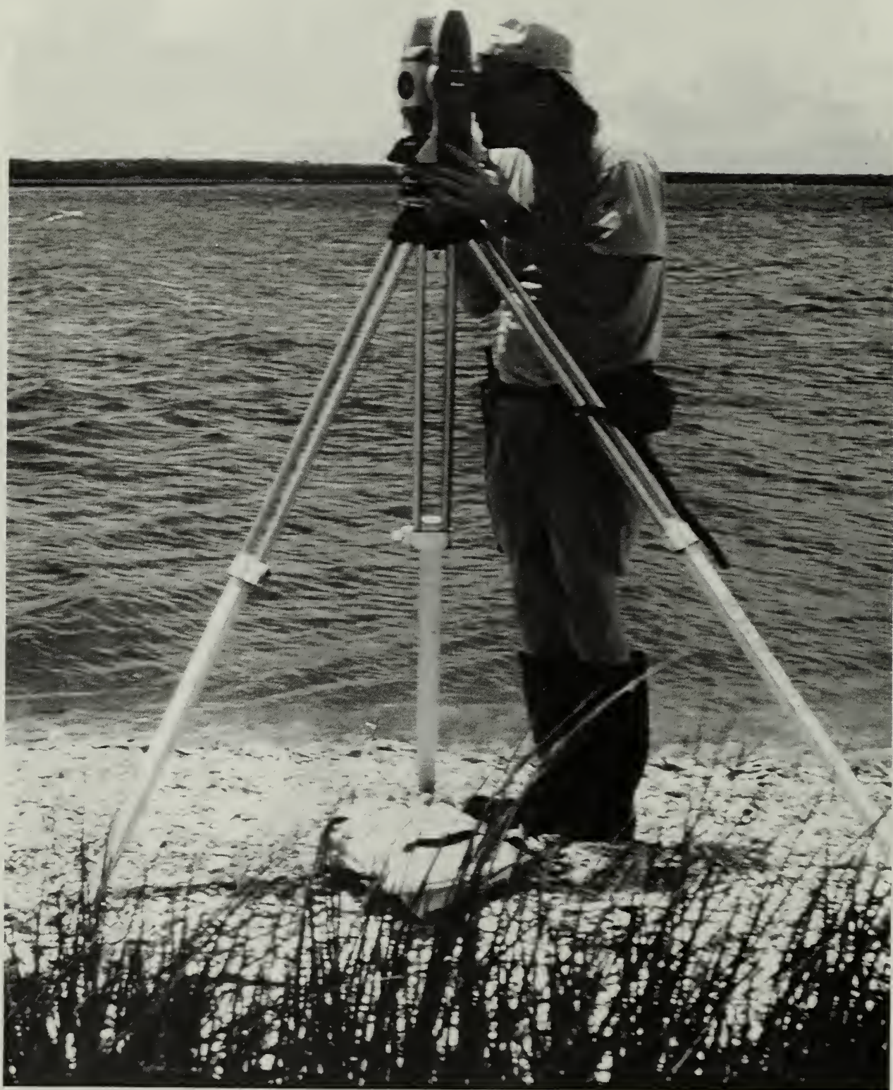
Figure 7. Sighting with Electronic Distance Meter to Prism Cluster
