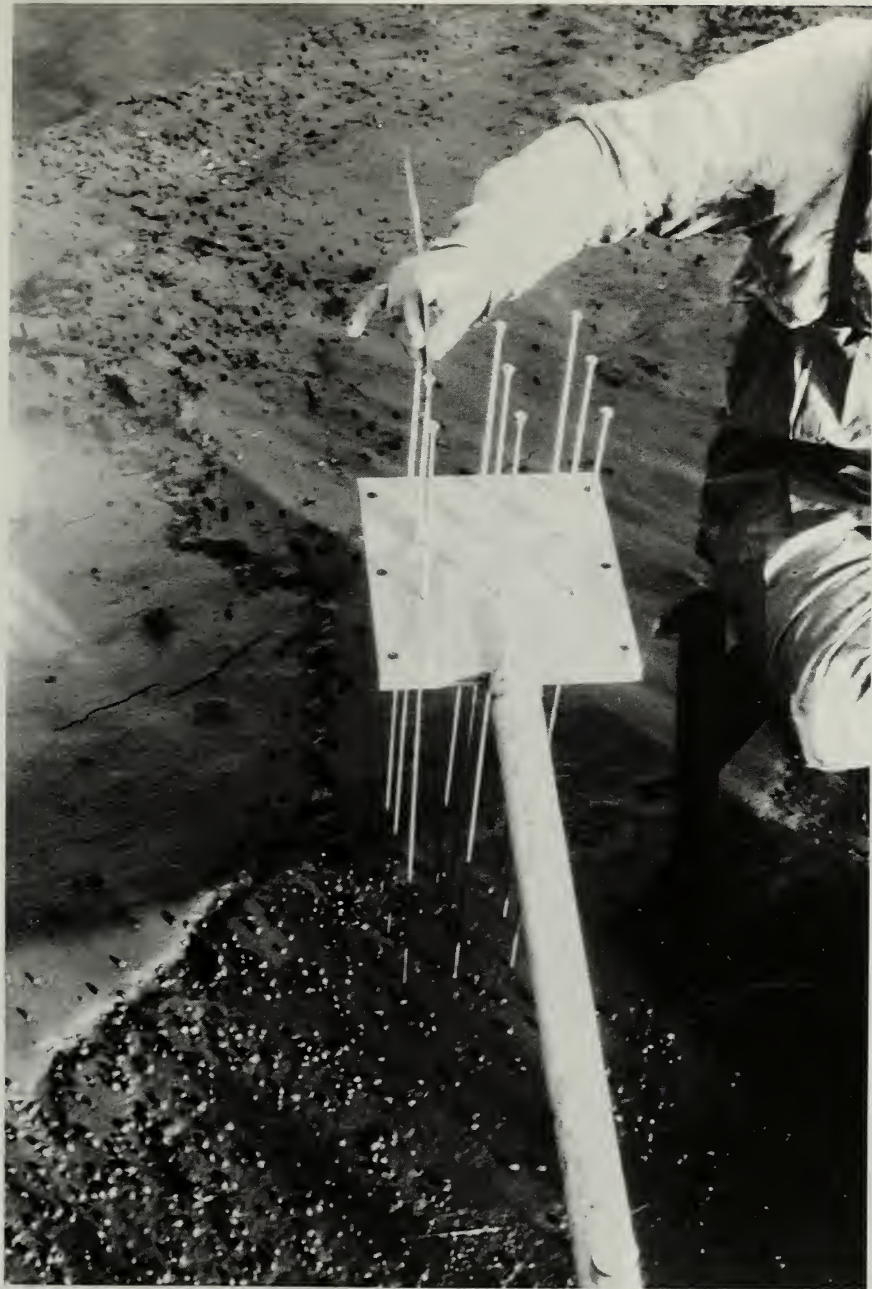
Figure 12. Sedimentation Table Measurements of Mudflat Surface
