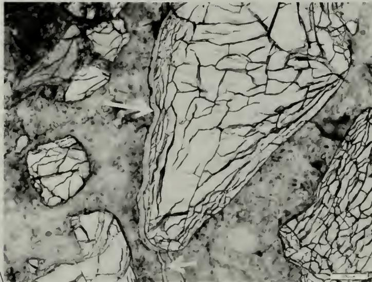
**Figure 2: Peripheral Fragmentation of Quartz with Cracks Extension (arrows)**
