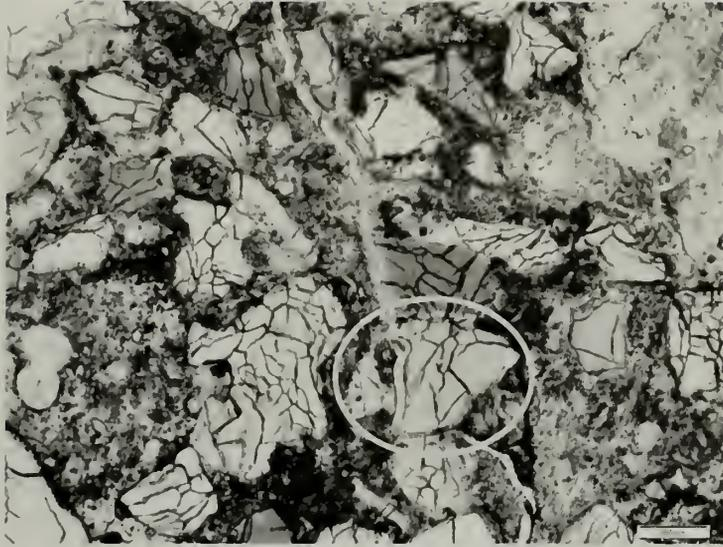
**Figure 4: Fracture of Quartz Grain in Core 6-1-25 (circled)**
