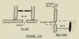
FIGURE 8 Relation of floor and wall vents to bins, House A.
