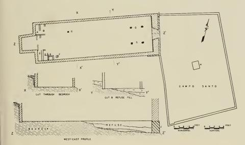
FIGURE 17 The church of Son Isidro, plon and sections, and the composanto. A, C, closetlike enclosures probably serving os sacristies; B, probable side alter; D, wall of roised sanctuary area; E, base for stand or cupboard holding baptismal supplies; F, sacrorium; G, stane bases for upright roof supports; H, masanry base for a cross in the camposanto; J, foundation—it occurs only at the east end of Son Isidro.
