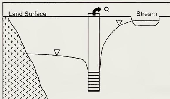
Drawdown in an aquifer bounded by a recharge and barrier boundary
