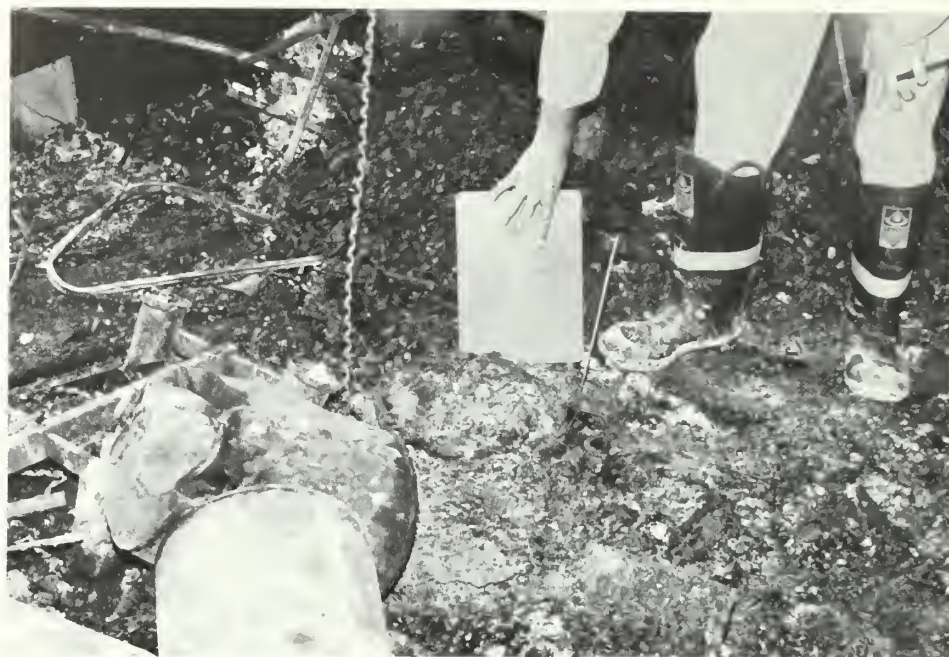
Figure 1. The spontaneous combustion of cloth rags that had been used in applying a common finishing wax caused over $1 million damage to a historic government office building in 1991. Remains of the trash can where the rags had been stored overnight is indicated by the fireman's notepad. After the cause of the fire was determined, a standard specification provision was developed for future contracts requiring the contractor to remove all material contaminated with finishing products from the site at the end of the day.
