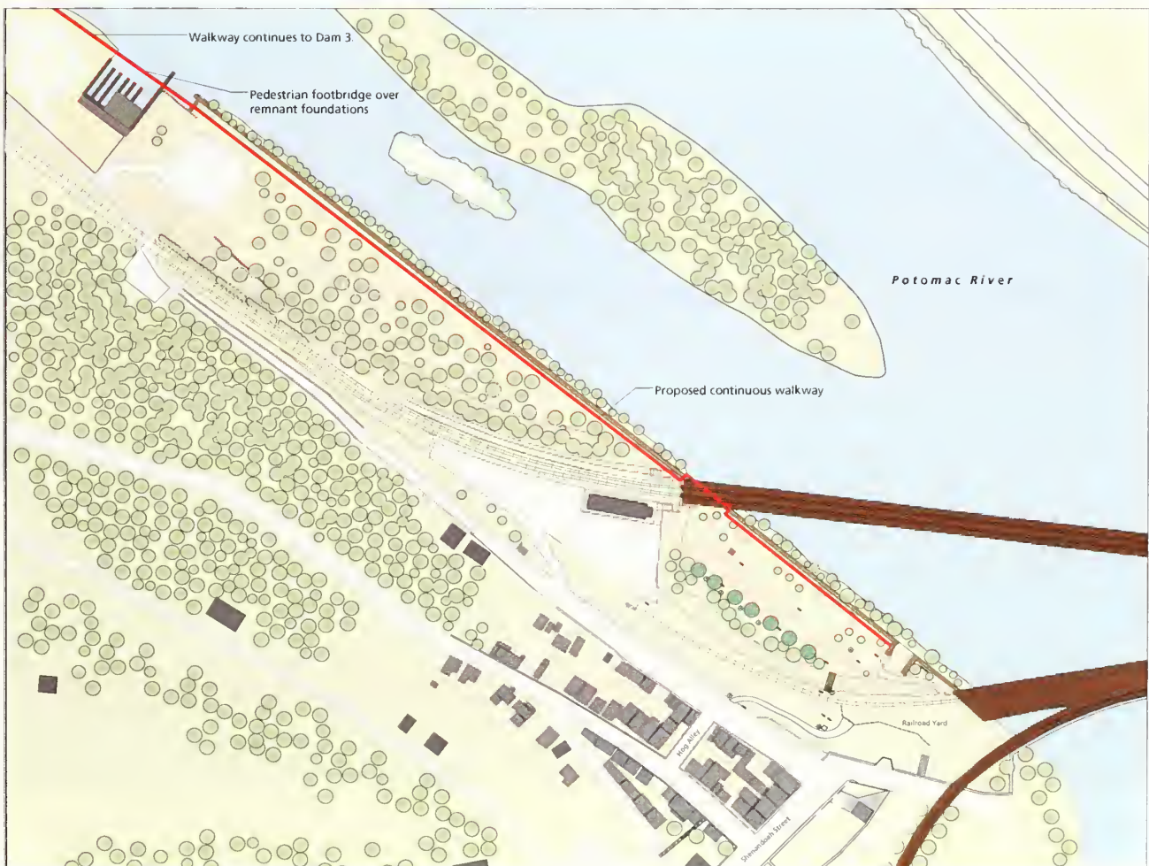
Figure 4.6. Diagram illustrating proposed continuous walkway, in red, from Lower and Upper Armory Grounds and beyond to the Dam. A cantilevered segment will be required under the railroad bridge to maintain continuity. OCLP, 2009.
