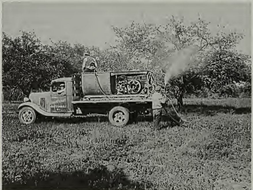
Figure 3.35: Historic photograph of spraying in an orchard in 1935 using a truck-mounted spray tank and powerful spray gun, Hightstown, NJ (courtesy of Library of Congress Prints and Photographs Division, Farm Security Administration, Office of War Information).
