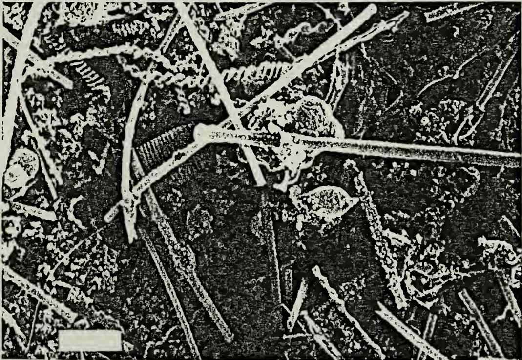
Figure 32. A scanning electron micrograph of the bacterial mat from dive 179. The scale-bar is 10  $\mu\text{m}$  in length. The genus, *Gallionella* are the forms with twisted sheaths; *Leptothrix* are the straight sheaths. The ribbed dome-like form in the center is thought to be a protozoa. This form is seen on many of the SEM photos and could be feeding on the bacteria. The tube-like form in the center-right with a blunt end is part of a diatom.
