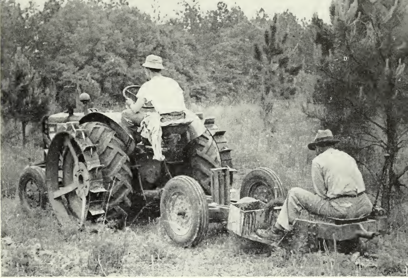
Fast, labor-saving mechanical tree planters are aiding reforestation in Georgia.
