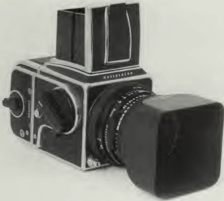
6 x 6 cm Single-Lens-Reflex Camera with lens shade. (Frederic Athearn, 1995)
