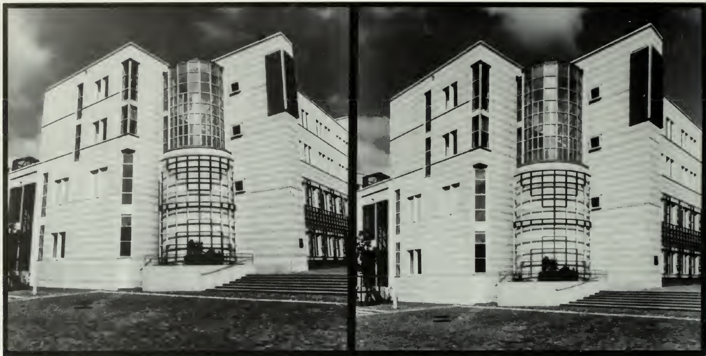
The photo on the left was taken using a Zeiss Distagon 60mm lens. The one on the right was taken with a Zeiss Distagon 40mm lens plus Zeiss PC-Mutar 1.4x Shift Converter for Hasselblad. Without the PC lens the building appears to be leaning backward. (Photos courtesy of Hasselblad, 1990)
