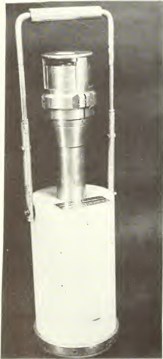
Figure 4.--Quick-release cable clamp installed on the shield and standard.
