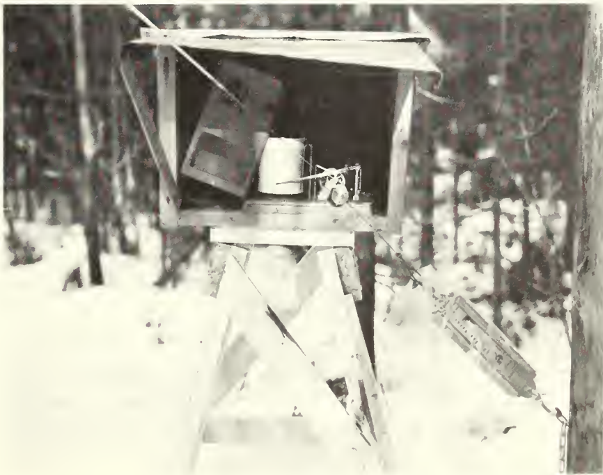
Figure 2. --Closeup of the recording apparatus and spring-tension scales.
