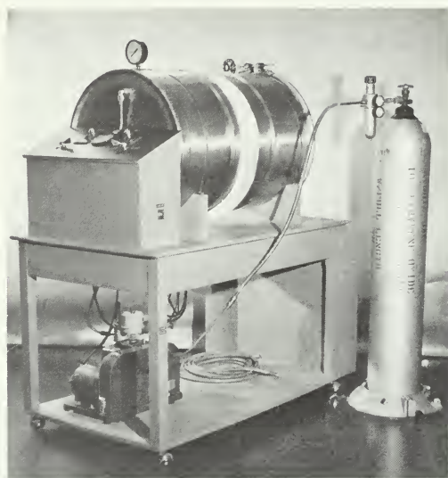
Figure 3. This fumigation tank was designed and assembled by the National Park Service Division of Museum Services. The tank permits fumigation under vacuum, at normal atmospheric pressure, or with moderately elevated pressure; and at room temperature or up to 180° F. (82° C.). The unit includes safety and monitoring devices.
