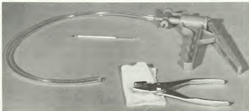
Figure 14. Testing kit for pollutant gases in the air. The device measures amounts of sulfur dioxide, nitrogen dioxide, hydrogen sulfide, carbon monoxide and carbon dioxide in parts per million.
