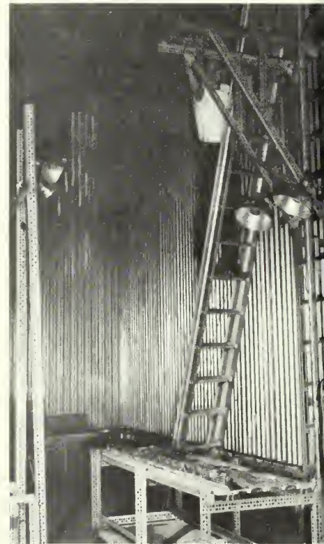
Figure 3.--Fuels: A , Measuring out 1-pound increments; B , Building up a fuel bed; C , Hoisting tray into wind tunnel throat; D , Photographing burned fuel bed.
