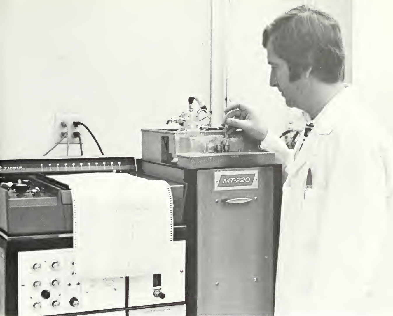
Tissue residues of lampricides are determined by gas chromatography in order to determine rates of uptake and release by fish. Photo by L. L. Marking.
