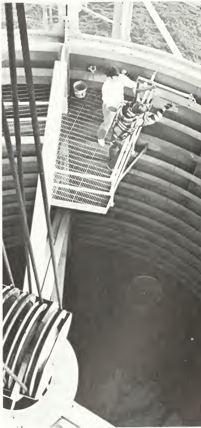
During the generation of electricity at the Jocassee pumped storage hydroelectric plant in northwestern South Carolina, water flows down through 40-foot-diameter penstocks from Jocassee Reservoir to Keowee Reservoir. Plankton nets placed about 45 feet deep inside these conduits measure the loss of young fish.
