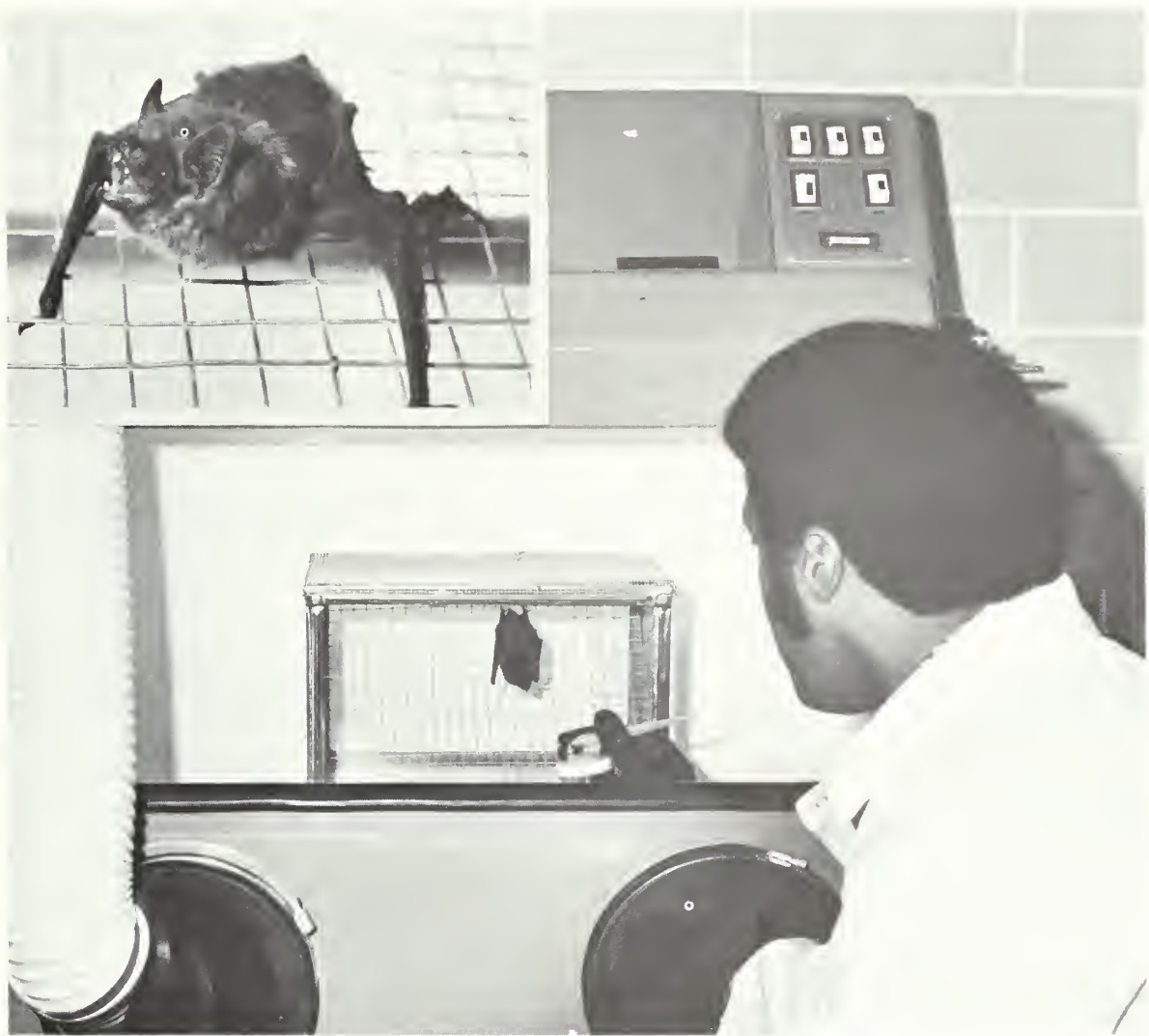
A repellent-test chamber used to assess the effects of nonlethal chemical aerosols upon the behavior and physiology of little brown and big brown bats. (Insert) A close-up of a big brown bat. Photo by Ray T. Sterner.
