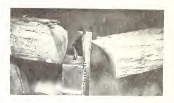
Figure 1.--Buckled thin shear blade after crosscut shearing a 6-inch diameter oak bolt. Blade thickness is 1/8-inch B/A ~ 1.0.
