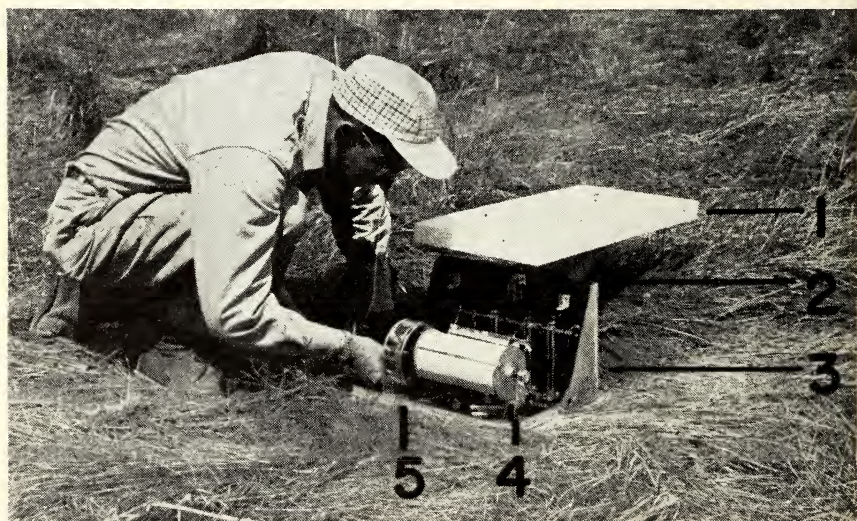
FIGURE 1.—Dew gage with block of expanded polystyrene in place, and the cover removed for adjustment of the balance: 1, Expanded polystyrene dew block; 2, support; 3, base; 4, drum and chart; 5, 7-day-clock drive.
