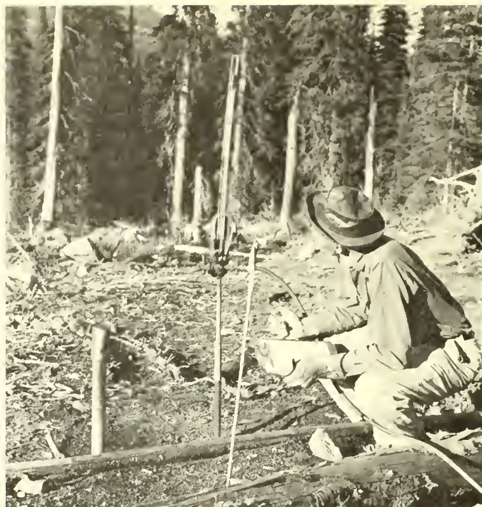
Figure 1.--Measuring hydraulic conductivity on the Elk Meadows research site, Idaho.
