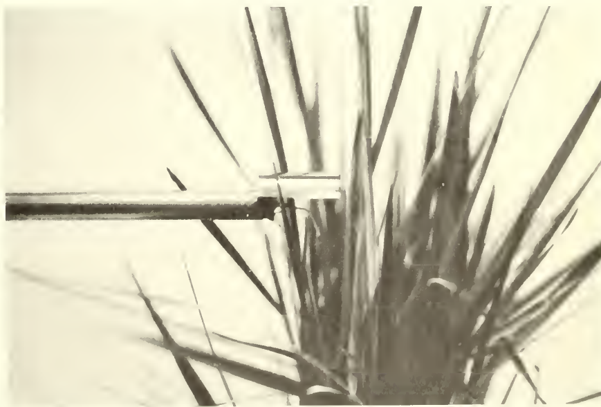
Figure 2.--The fine-wire psychrometer can be used in controlled-environment growth chambers, or in the field, to measure the relative humidity of the air within the canopies of growing plants.
