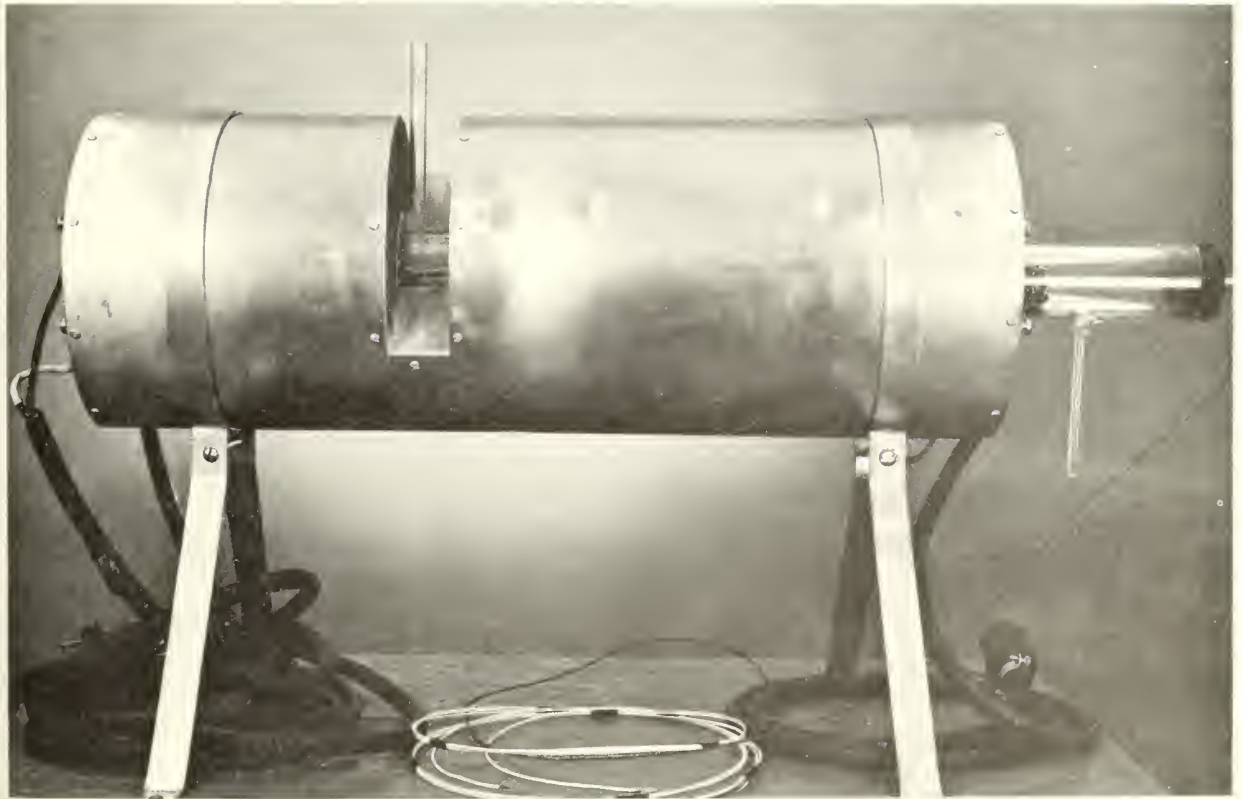
Figure 5.--Stainless steel covering and support assembly of furnace.
