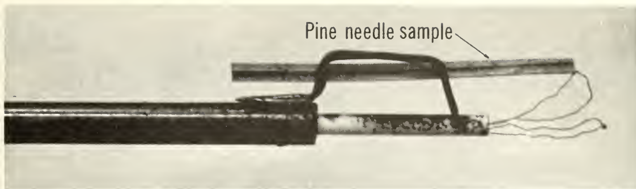
Figure 7.--Enlarged section of ignition boat with a 1-inch section of pine needle in test position. Note positions of air temperature thermocouple and surface temperature thermocouple.
