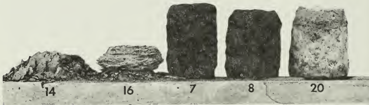
FIGURE 7. Selected cylinders subjected to freeze-thaw test. Nos. 14 and 16, with 10 and 12 percent cement by volume respectively, failed at the third cycle. Both were made up with equal parts clay and silt-loam. No. 20, with 15 percent cement by volume, is shown at the 12th cycle. Nos. 7 and 8, consisting of three parts clay, two parts silt-loam, and emulsified bitumen, were tested in conjunction with the soil-cement and are shown at the 15th cycle.
