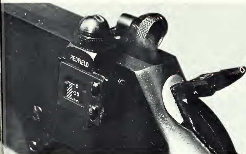
The aperture or "peep" sight is both sturdy and accurate. Its quick handling properties have established it as a long standing favorite with woods hunters.
