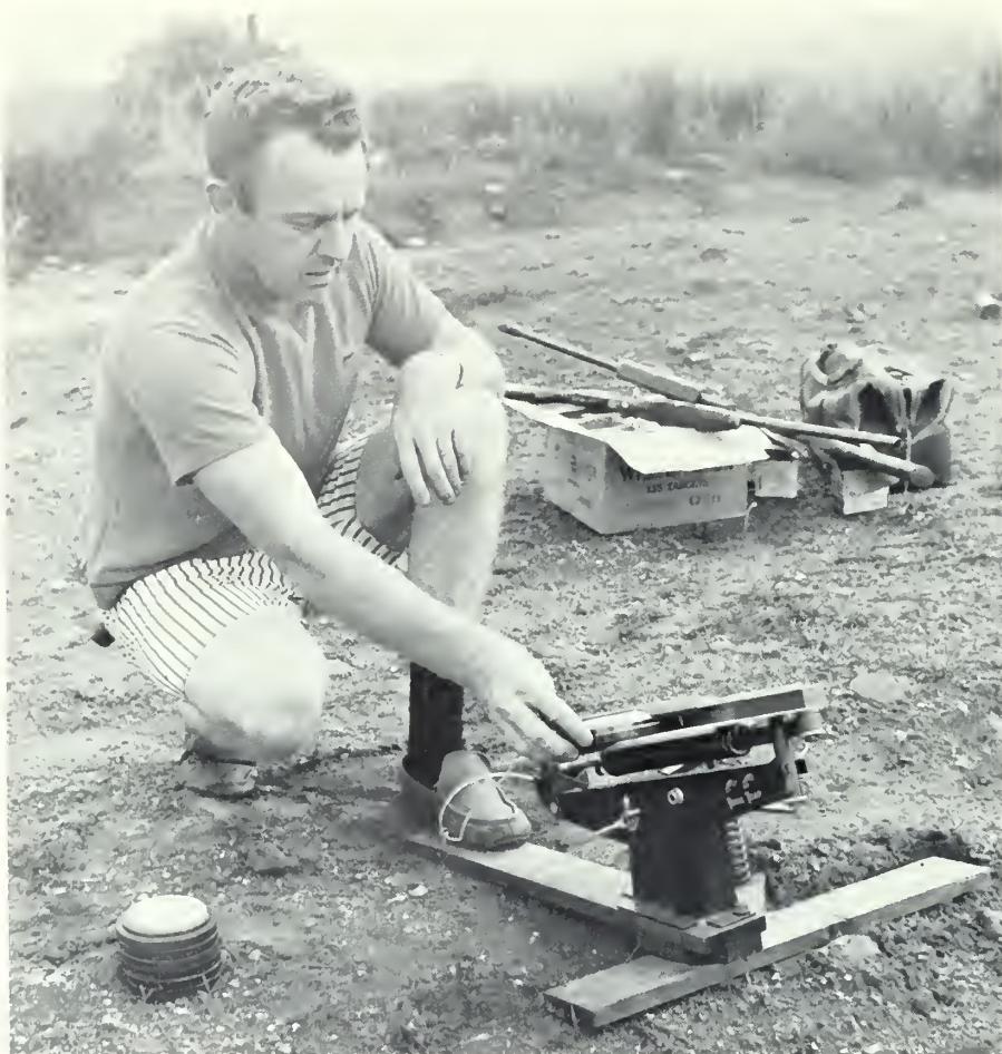
The direction which the target flies can be controlled somewhat by just where on the throwing arm the target is placed. The height of the bird can also be adjusted. This type of trap can also throw doubles and triples.
