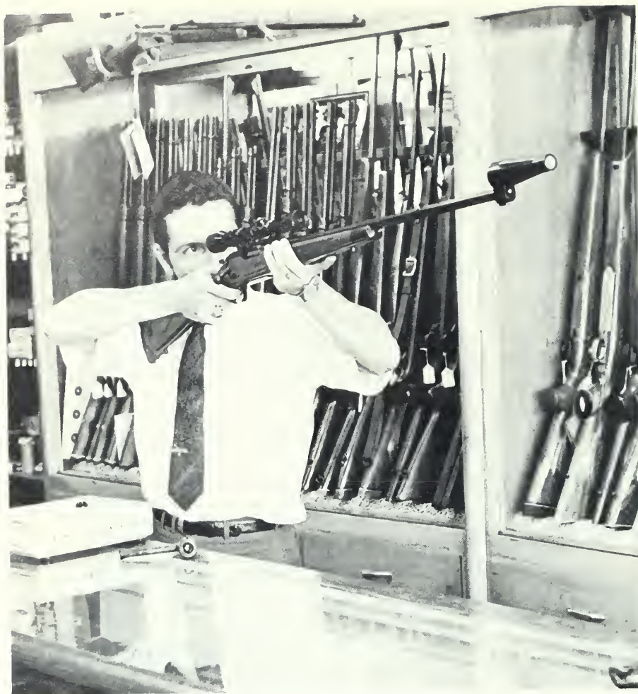
Dick Kennedy, of the Gunroom, lines up a scope by using a collimator. This device aligns the sights with the bore and can save the shooter a good deal of time and trouble. Once the sights have been collimated the rifle can usually be sighted in with only a couple of adjustments.
