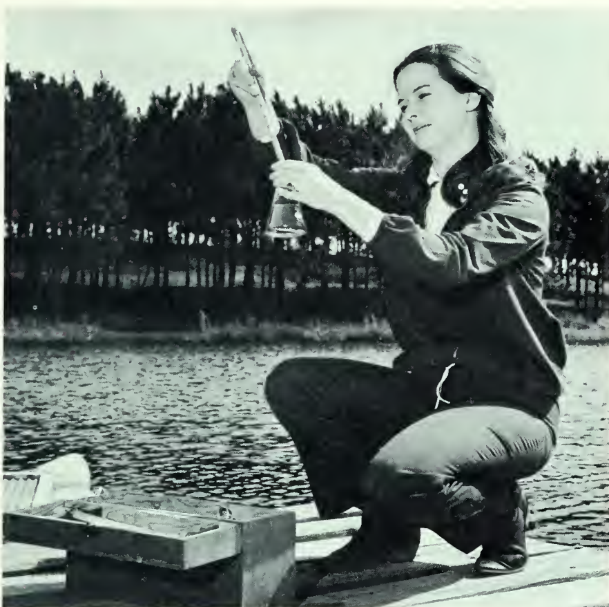
The author checks the oxygen level in a catfish pond by chemical analysis. Such testing is a necessity in commercial production.
