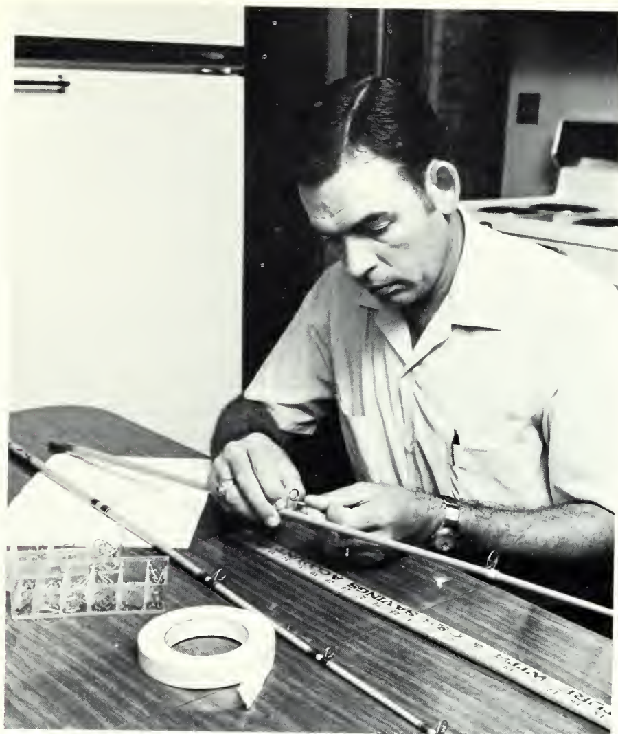
Rev. Bill Conine finds rod building almost as interesting as fishing. Here he spaces and tapes on the guides of a casting rod with the aid of a guide spacing chart.
