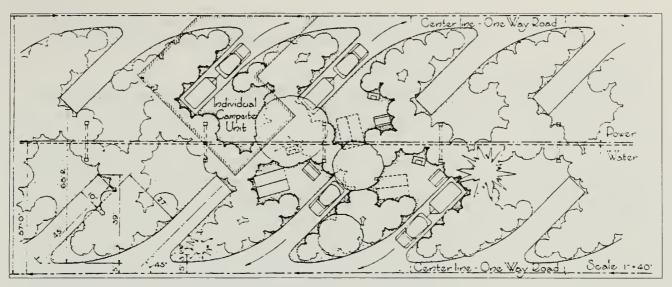
Figure 65. Good's drawing depicting two rows of angled spur campsites showing how adjacent campsites are screened using vegetation. (Albert H. Good, Park and Recreation Structures, 1938.)
