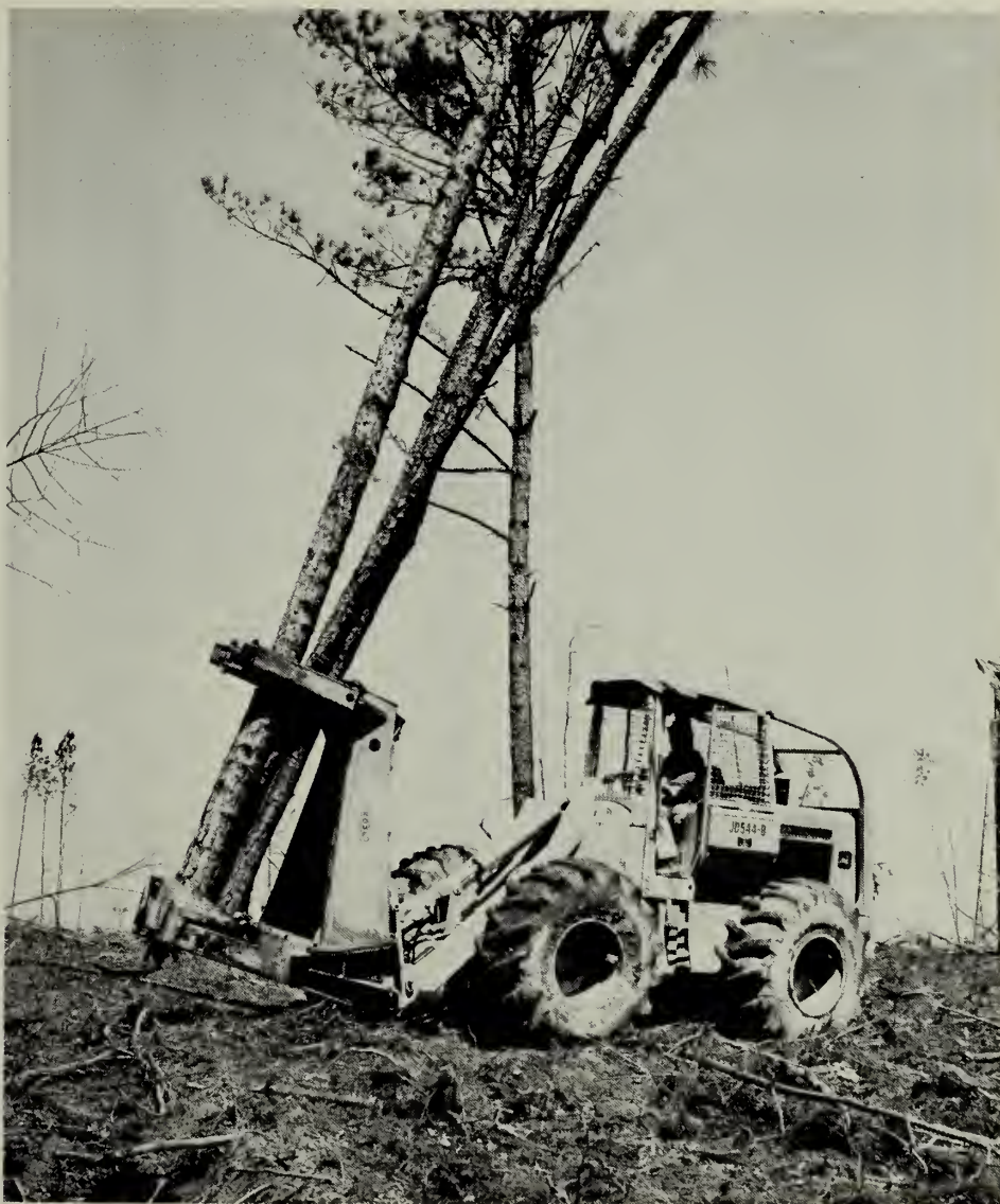
Fig. 2. A feller-buncher in a clear cut harvesting operation.
