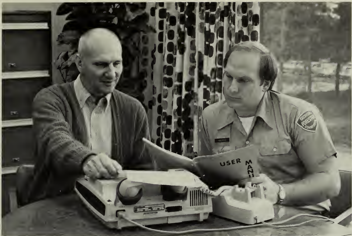
Figure 1 --An example of a computer terminal with built-in acoustical coupler, which can be used to access the Forestry Weather Interpretations System (FWIS).
