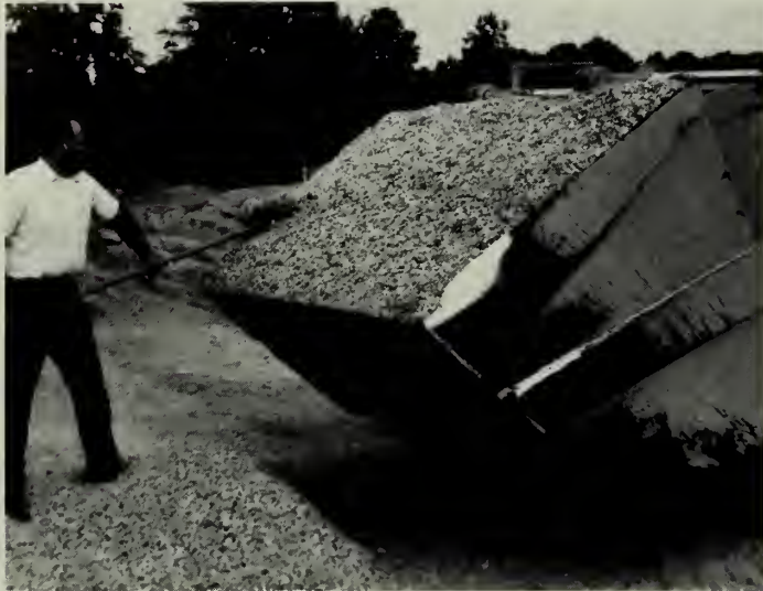
Figure 1. Leveling of front-end loader bucket filled with wood fuel.
