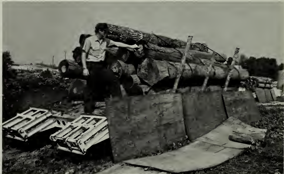
Figure 2. — The stored logs remained on trailers at the storage site throughout the study period. Baffling was done to prevent air movement under the logs.
