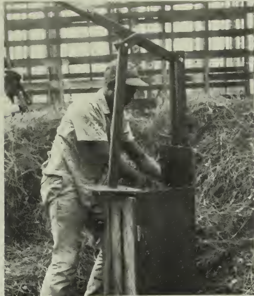
Figure 1: Pinestraw is commercially baled using either a box-baler (left) or a modified hay baler (right). Note the stack of loose pinestraw ready for baling.
