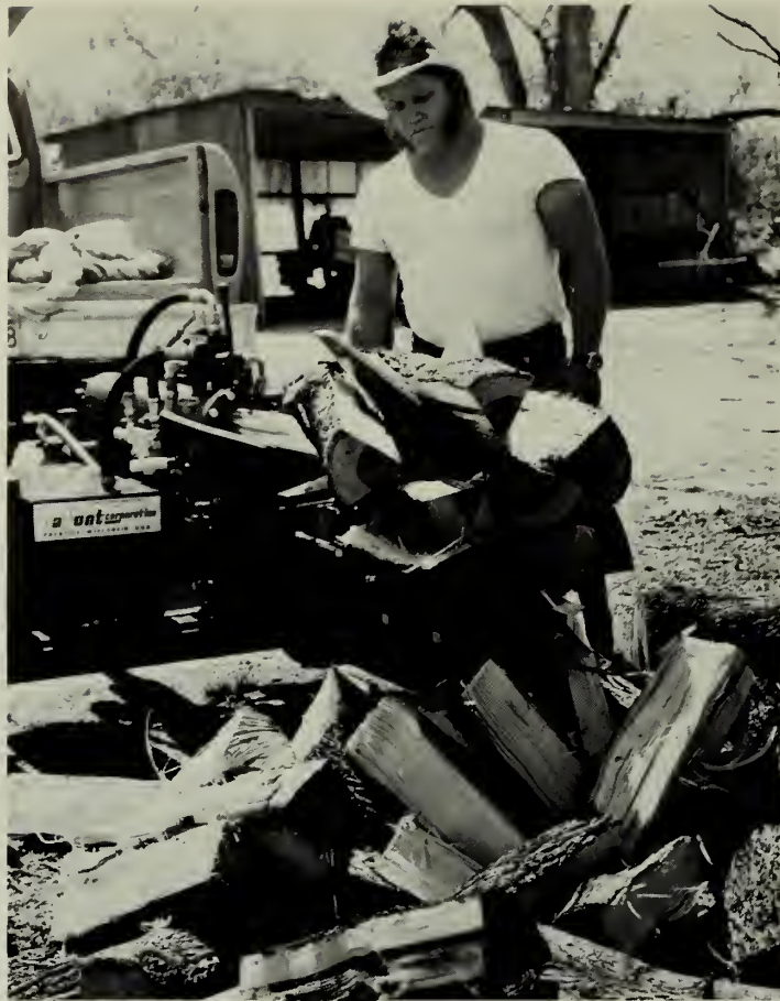
A woodyard owner operates an automatic splitter, one of the great labor saving machines that has been invented in recent years to make volume production possible.
