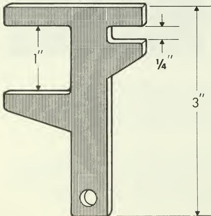
Figure 11.--A Go-No-Go gage can be cut from 1/16 or 1/8-inch sheet aluminum. Cut the notches slightly tight and file smooth to final dimensions.
