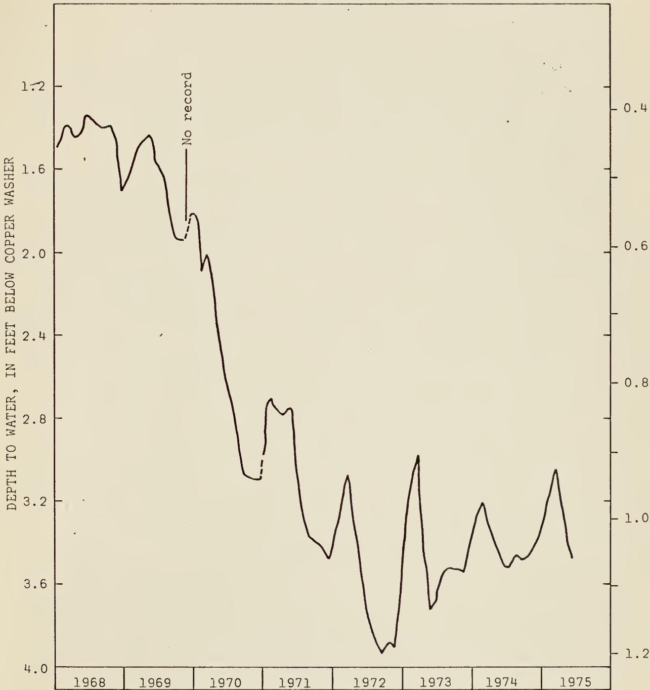
Figure 3.--Monthly low water levels in Devils Hole.
