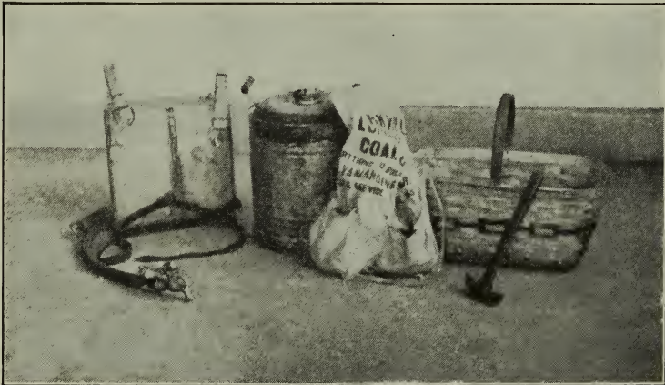
FIGURE 19.—Equipment used by a field distributing crew—distributing tank, can for temporary storage of poison, carpenter's apron, basket for unfilled paperoid cups and tops, and hammer.
