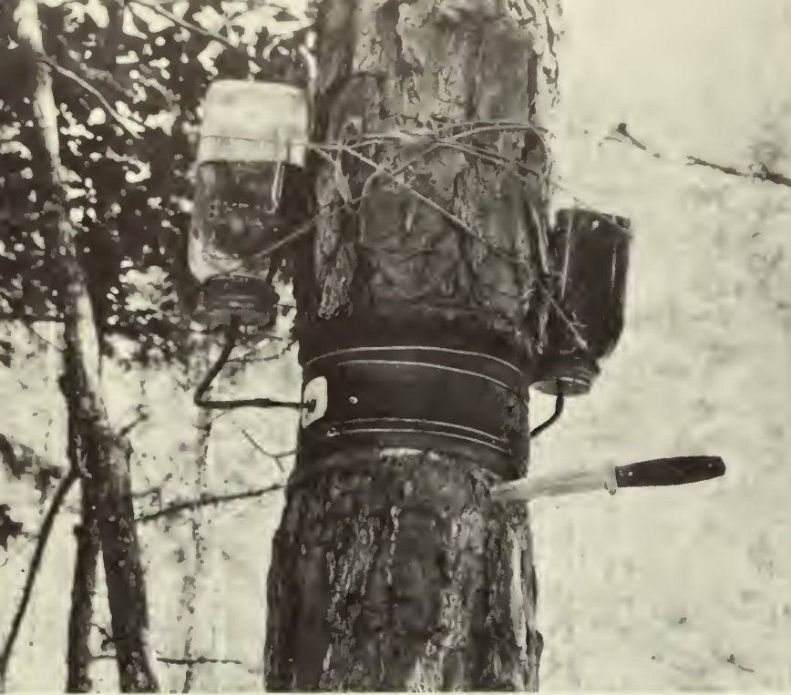
Figure 11. --Equipment used to inject chemicals into the sap stream of pines to control the southern pine beetle.
