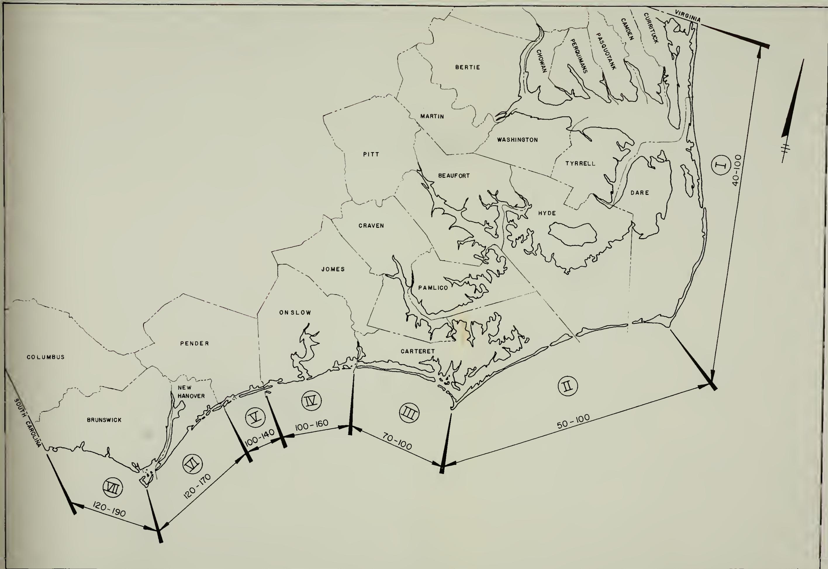
Figure 3. Recommended range of recession lines from the dune toe for one in twenty five years storm return frequency
