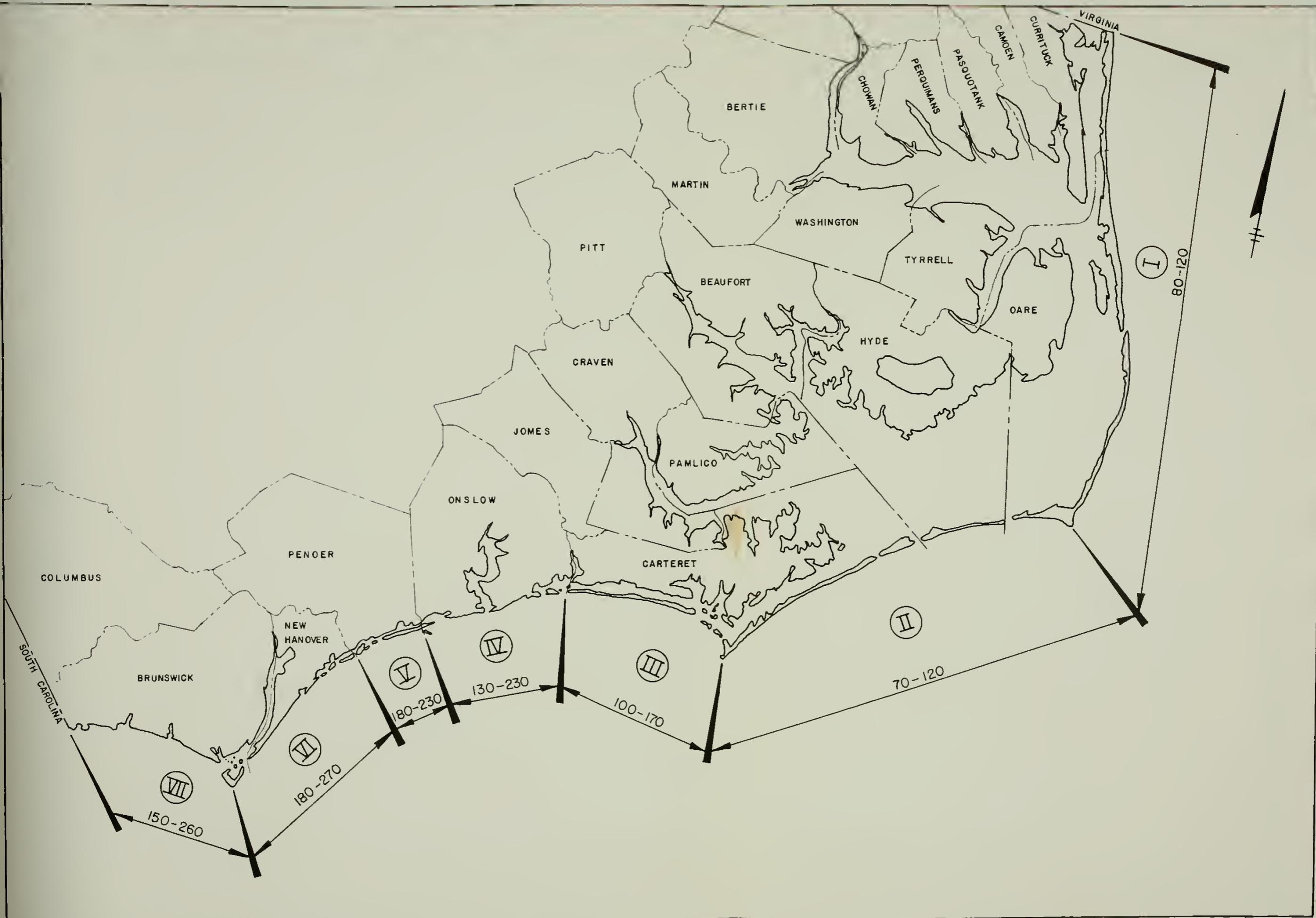
Figure 4. Recommended range of recession lines from the dune toe for one in a hundred years storm return frequency
