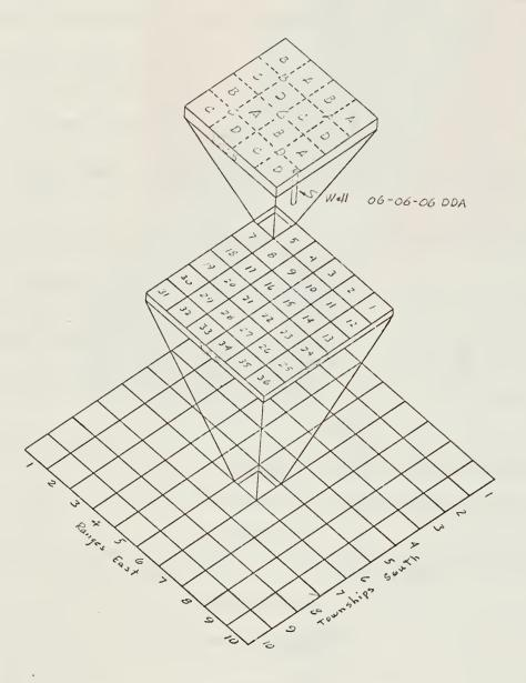
Figure 2.—Location-reference method of numbering wells, springs, and test holes.
