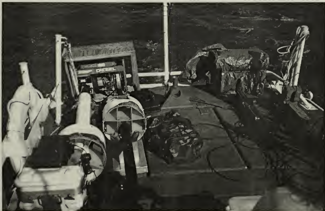
Figure 2. Survey instrumentation on the deck of the NPS-SCRU survey vessel. The magnetometer is on the left, the side scan sonar on the right. NPS photo by Tim Smith.
