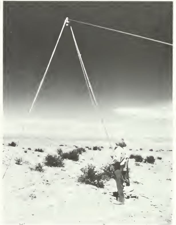
Figure 11 A bipod with attached 35-mm camera and guy lines over a small archeological site.
