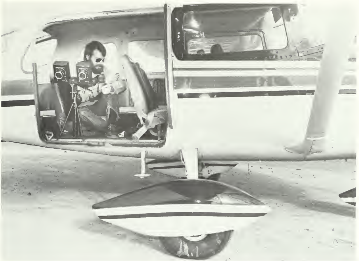
Figure 9 Photograph of do-it-yourself camera mount emplaced in the open doorway of an aircraft.
