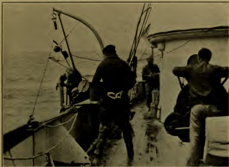
FIGURE 1.—Oceanographic work aboard the U. S. F. S. Albatross II . One of a series of Greene-Bigelow water bottles with a sample of sea water from a known depth is being brought aboard.
