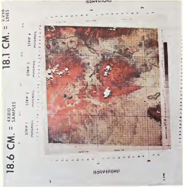
Plate 7 Demonstration of the use of pixel overlays to aid in precise coordinate location on Landsat images. Courtesy Technology Application Center.
