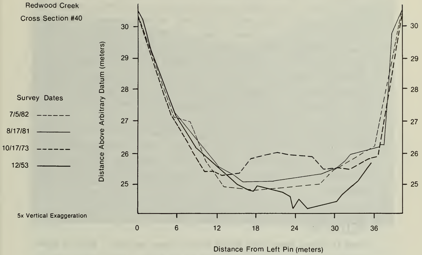
Figure 9: Cross Section at the U.S.G.S. gaging station on Redwood Creek near Blue Lake. Cross sections at or above this location have shown persistent scour for nine years.
