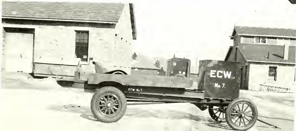
ECW No. 7 portable engine mounted on trailer. Box in front is for tools and spare tires. (Picture taken before safety device was installed.)
