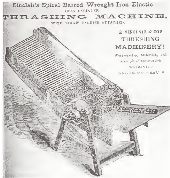
Figure 11. Thresher. This “Thrashing Machine,” typical of the period, threshed the grain, separated it from the hay, and then separated the grain from the chaff as the grain fell to the floor and the chaff was blown away. (Smithsonian Institution)
