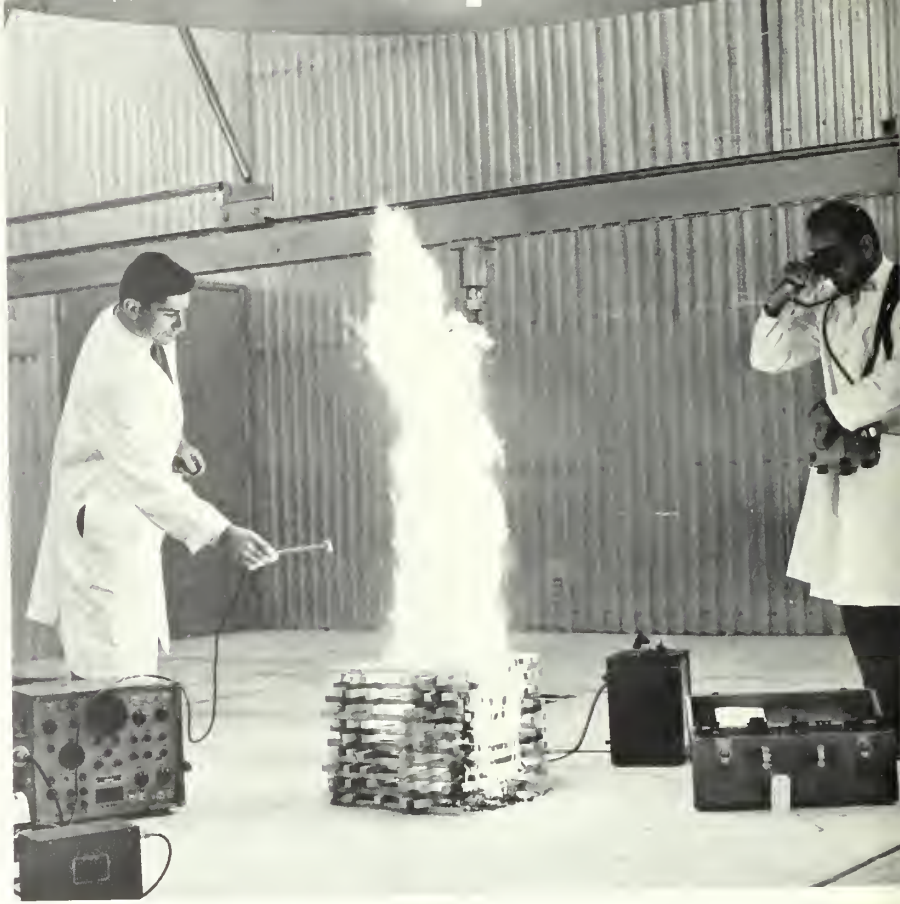
Temperature and updraft speed of crib fire is determined in combustion room
