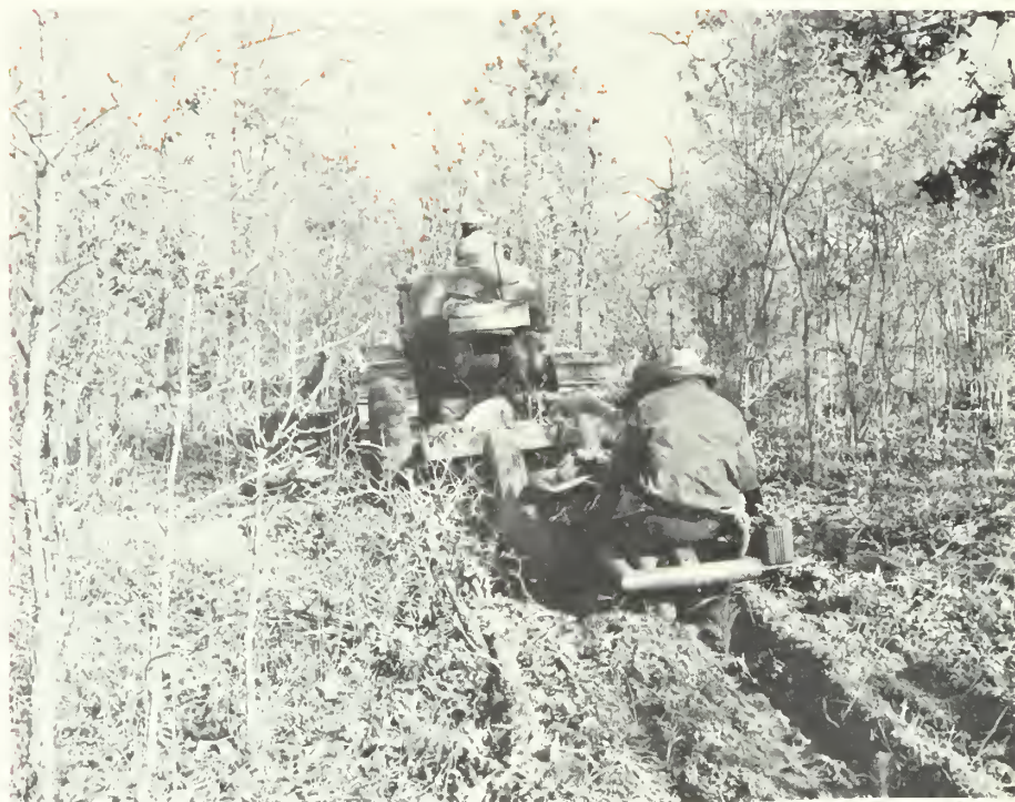
Tractor-train serves a two-fold purpose for E. G. Gragg. A beam in front clears away the scrub oak as planter in rear puts in slash pine.
