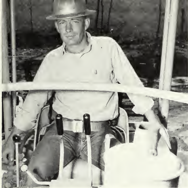
Seat belts, along with brush guards, have increased the safety of Commission tractor operators.
